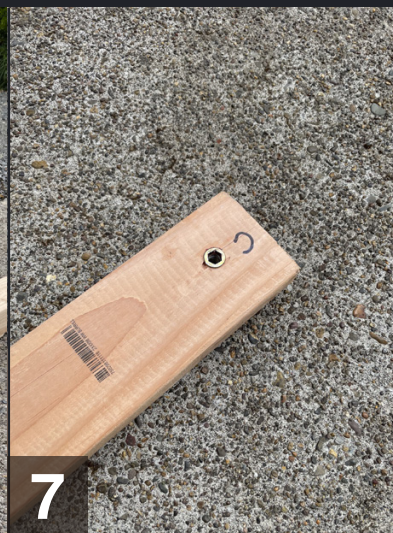
7 Rear Bolts enter from the rear and connect to threaded inserts in beams.
