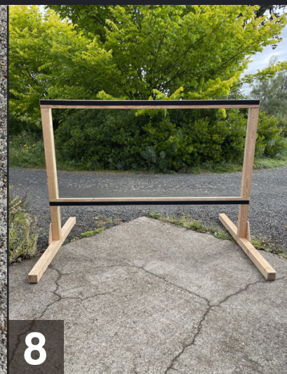
8 Assembled Stand is ready for screen mounting with male (non-fuzzy) hook-and-loop tape on top and bottom beams.
